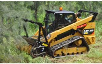
The Magnum Mulcher is the perfect for clearing firebreaks, land clearing, maintenance of park or forestry trails, utility line clearing, vegetation management and re-mediation. Suited to High Flow Skid Steer Loaders & Excavators up to 20 tonne the Mulcher is ideal for grinding small and large material, trees or brush up to 8" in diameter.
