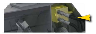
Bi-directional flow manifold with cross-over relief allows the operator to direct debris away from bystanders, other machinery, and buildings
